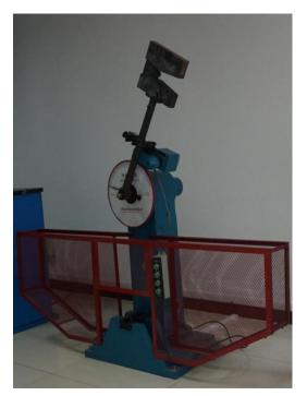
Features: The pendulum impact and after impact left before the potential energy difference displayed on the dial of the way, get absorbed energy of sample.
