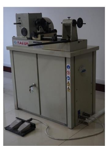
**Features:** Samples in the absence of any torsional per second does not exceed a circle of constant velocity along the direction of a helical line tightly wound on the mandrel, the equipment can according to requirements, test solution of circle or circle solution and wound; specimen diameter: 0.50 mm  $\sim$  6.00 mm, winding speed: 15 r/ min , 20r/ min, 60r/ min.
