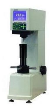
**Features:** LCD display; Menu operated LCD screen with good operability and readability; Digital LCD reading of 15 regular hardness scales and can convert to all other hardness scales such as Brinell, Vickers, Rockwell and Rockwell Superficial; Integrated printer for test result and RS232 data output to computer. Maximum allowable sample height is 170mm.
